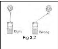
**⚠** Do not winch from an acute angle as the wire rope will pile up on one side of the drum causing damage to wire rope and the winch. Fig 3.2
